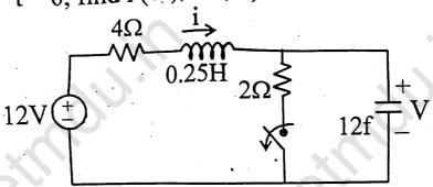
5. Find V(t) for  $t \ge 0$  in the RLC circuit as shown in fig. below:
